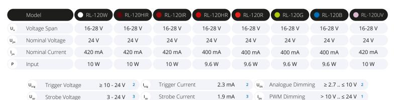
1 PWM maximal rate is ≤ 40 kHz 2 EN (Enable) trigger signal values, M8 connector – pin number 4 3 Driving voltage and current M8 connector - pin number 2
